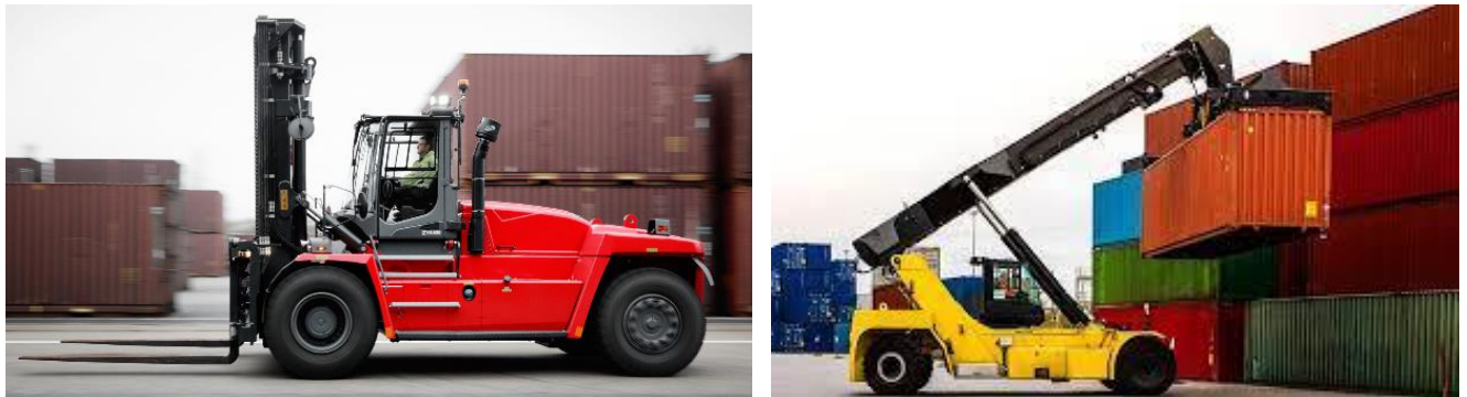
Figure 3: A Type of Forklift (left side) and Stacker (right side) Used in Shipping Industry
