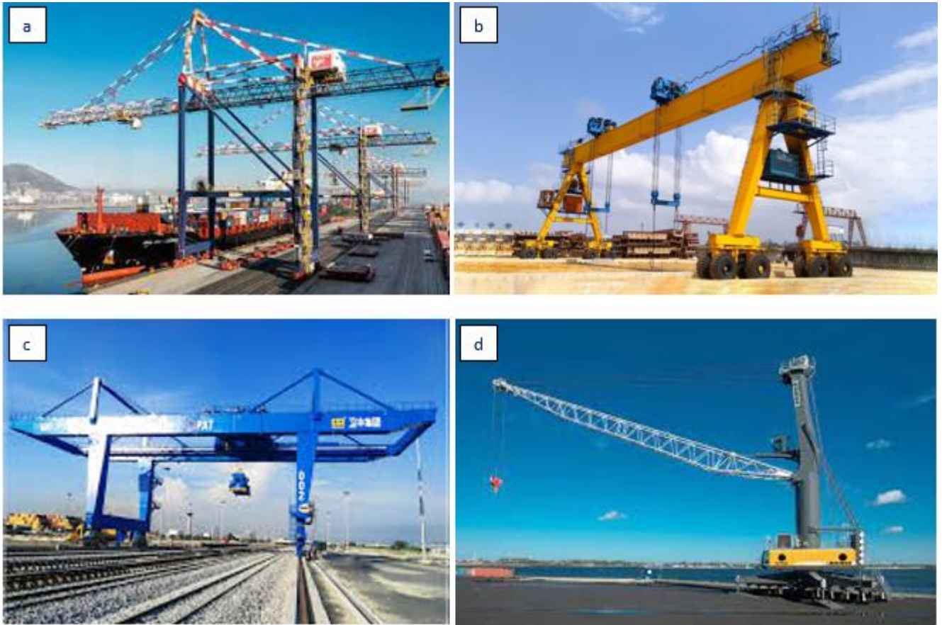
Figure 2: Different Types of Port Cranes: a) STS Cranes, b) RTG Cranes, c) RMG Cranes, d) MHCs
