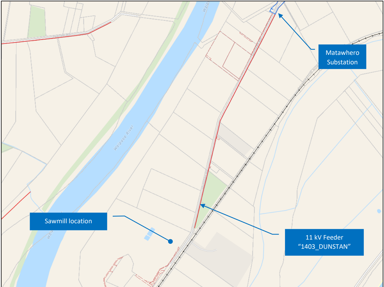
Figure 19: Gisborne Greenfield and Local Electricity Infrastructure
