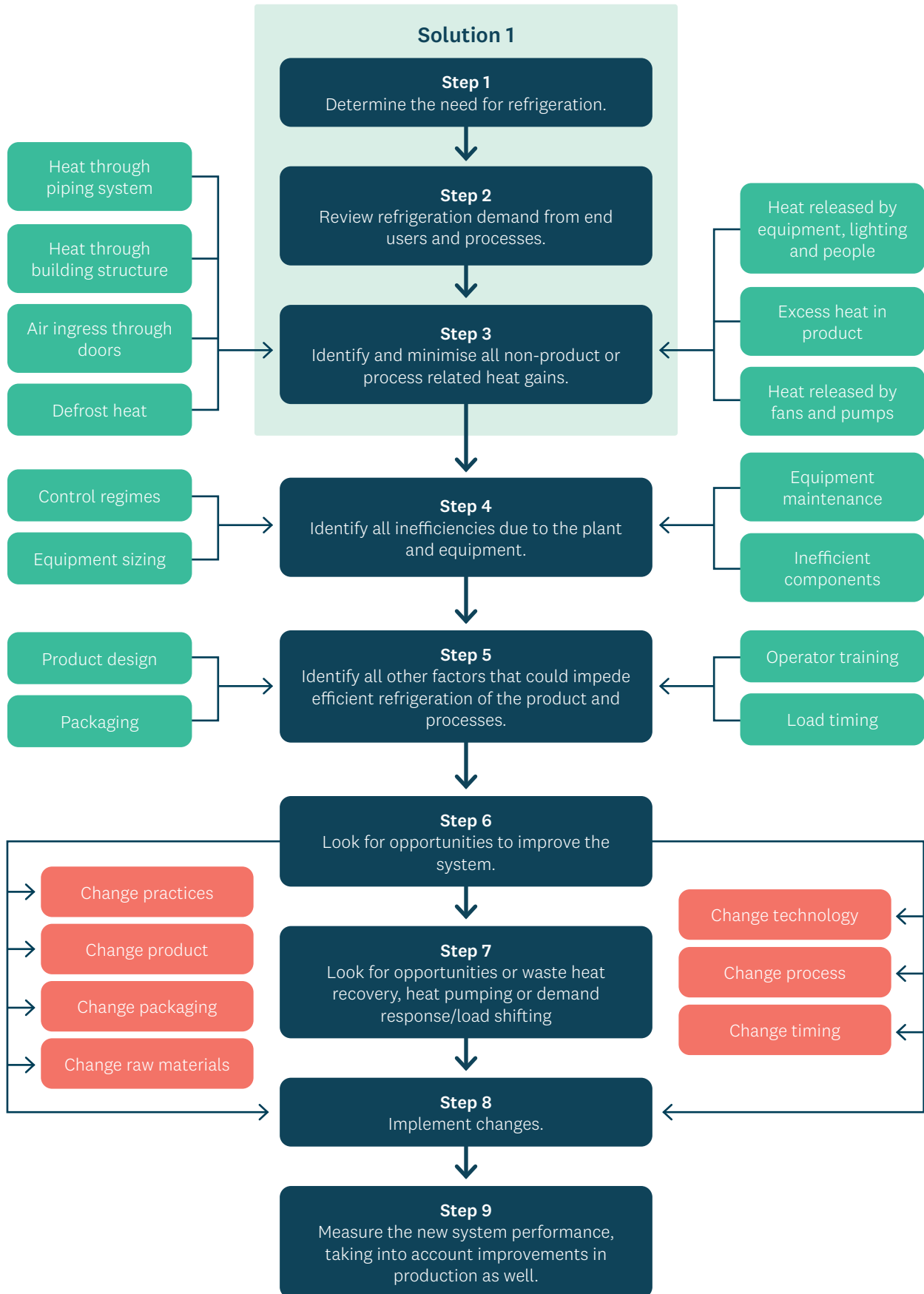
Figure 2: Steps identifying energy efficiency improvements in an existing refrigeration system
